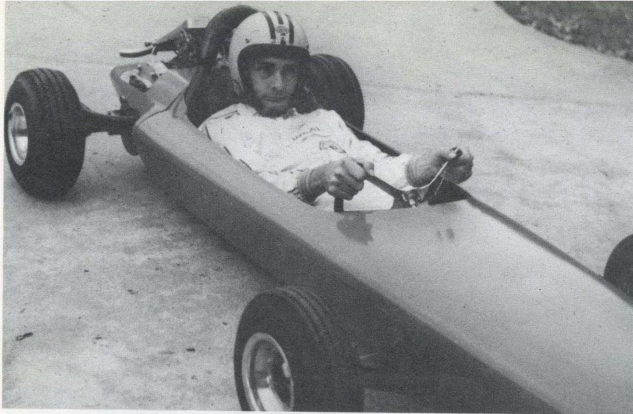
F/5 body shell is from a flawless mold. . . chassis is fully suspended.
