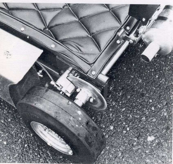
Red Devil boasts stopping power by Hurst/Airheart 6" hydraulic discs.
