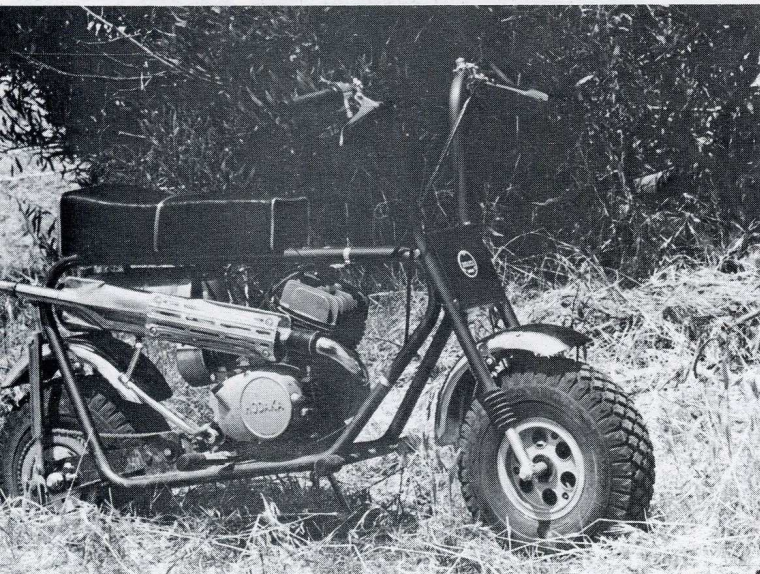
A Hodaka 100cc mill makes a mighty brute of the already rugged Bonanza mini-bike.
