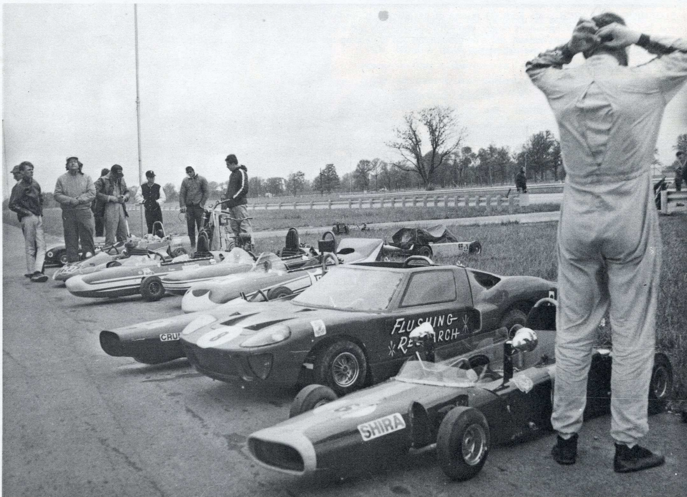
The nine FKE-I & II machines were combined with a sizable field of B-Limited enduro karts. Quite a variety of configuration here...one huge spoiler, an "open-legger" with exterior pedals, a sleuth-nosed FKE-II from Ohio with a home-crafted 2-speed arrangement on an 820 West Bend, and a maroon Ferrari, scarcely visible behind all the legs.
